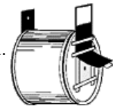
Pinhole camera made from a can.
