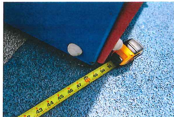
Use Zone - Inadequate at 4ft. to Labyrinth - CLASS B HAZARD
