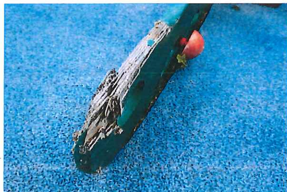
Crocodile Climbers (2) (Kompan) - Wood damaged, cracked & splintered - CLASS C HAZARD
