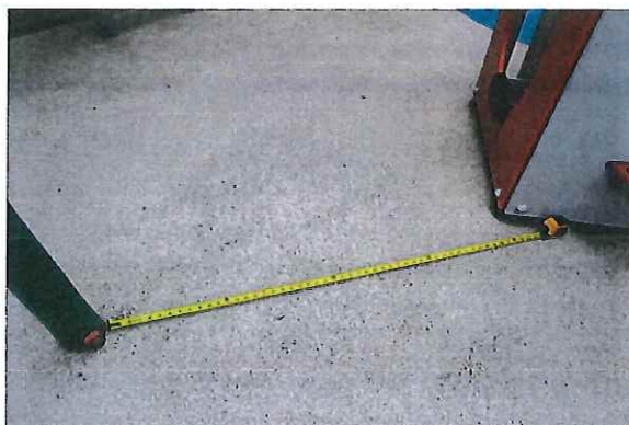
Use Zone - Inadequate at 4ft. on one side, overlaps w/ Labyrinth - CLASS B HAZARD
