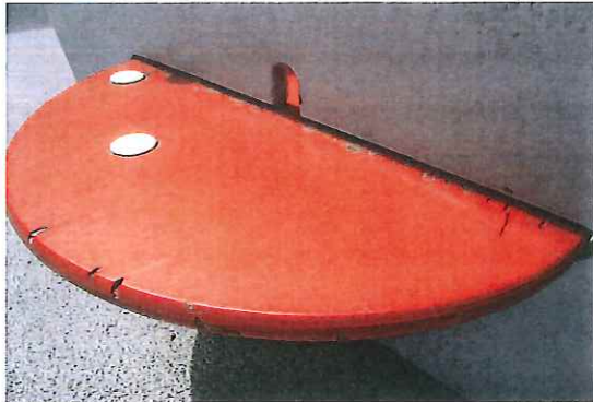
Spica GXY 8015 - Surfacing is peeling - MAINTENANCE
