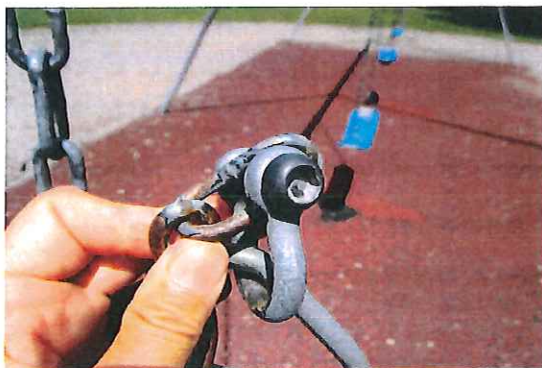
11ft. Swing Set (Unknown) - All chains worn - CLASS A HAZARD
