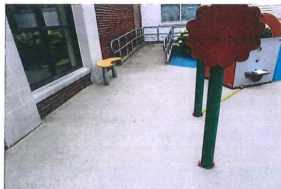
Use Zone - Inadequate at 4ft. on one side, overlaps w/ Labyrinth - CLASS B HAZARD
